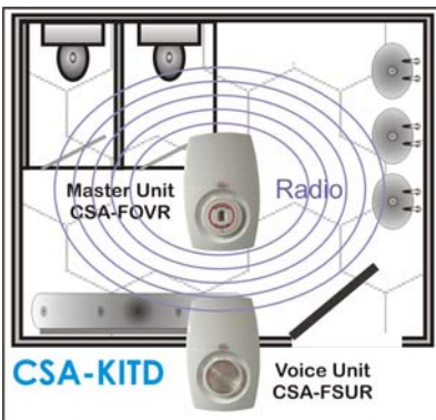
A Wire-Free kit Containing: 1 x Wire-Free Flame Detector Unit 1 x Wire-free Voice Sounder Beacon
